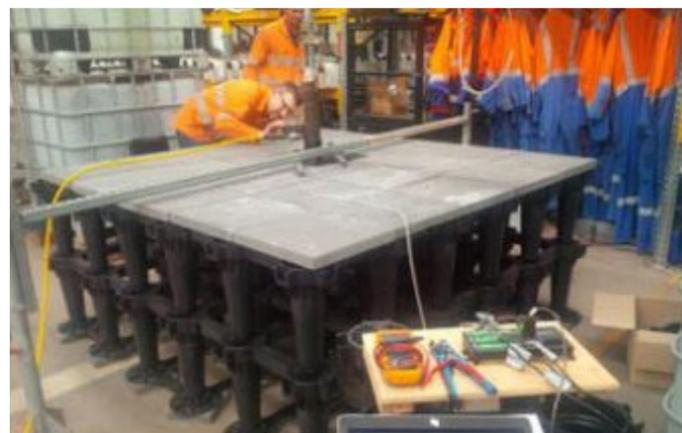
Figure 4.22 Strata Vault Cell Sample
